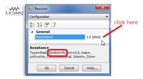
You can also view all the parameter symbols of a component by viewing the "Properties"
