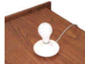
Load voltages are connected to load and flicker or power quality measurements are taken and tested for acceptability
