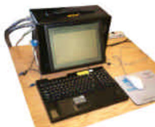
RTP used to simulate and record voltages and currents for real time playback.
