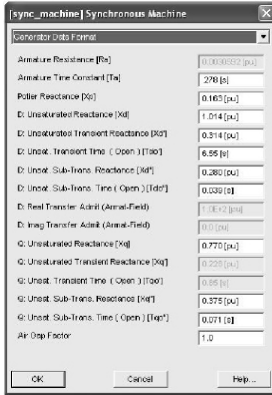
Figure 7-T3 - The 13.8 kV, 120 MVA Generator Parameters
