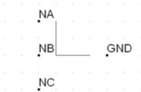
Figure 5-5 – Electrical Port Connections Defined in the Graphics Section of the Component Definition
